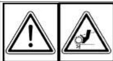
Caution! Never touch moving pulleys or belts. They can be very dangerous. Never do maintenance with engine running.
