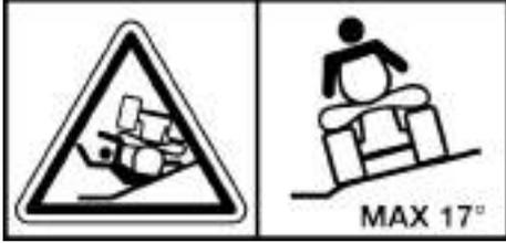
DANGER! Machine roll-over: Do not use this machine on slopes greater than 17° (30%).
