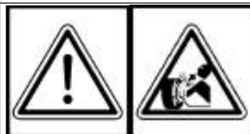
A burst which separates the tyre from the rim parts can cause serious injury or death.
